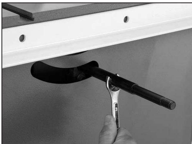
Figure 13. Installing the pivot shaft.
