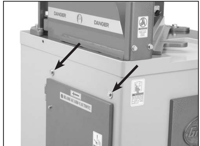
Figure 8. Bolts to be removed.
