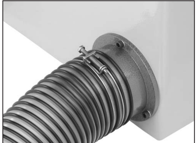
Figure 25. Flexible dust hose connected to dust port.
