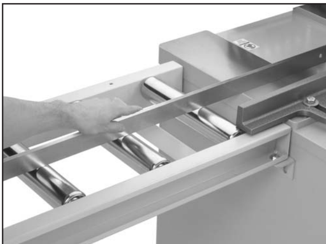
Figure 18. Using a straightedge to align the rollers even with the table.
