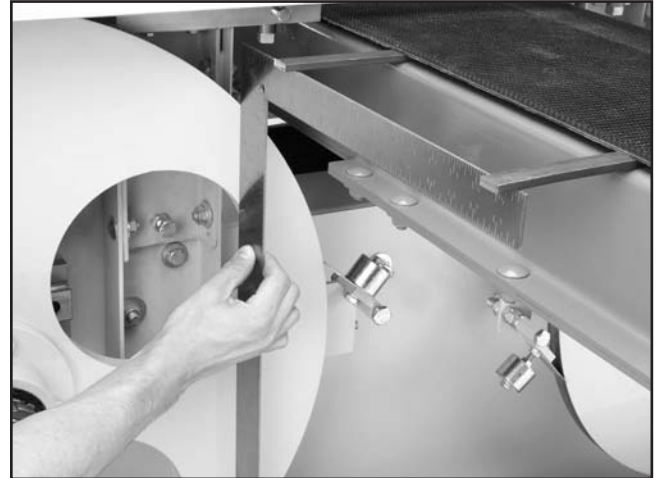
Figure 62. Checking table alignment.
