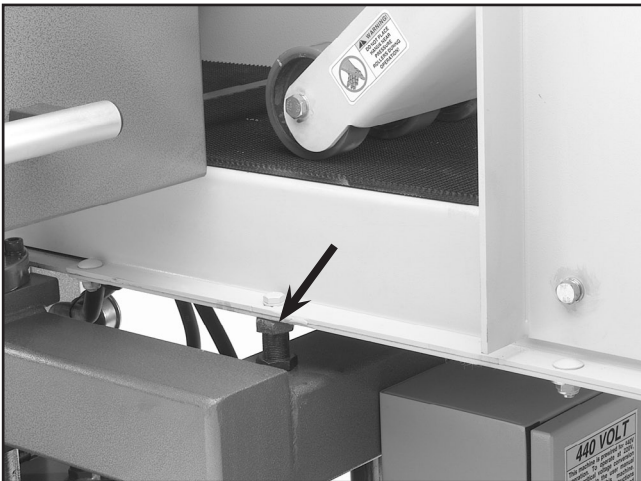
Figure 39. Conveyor table adjustment bolts (1 of 4 shown).
