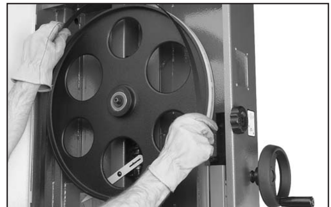
Figure 48. Placing blade on the wheels.
