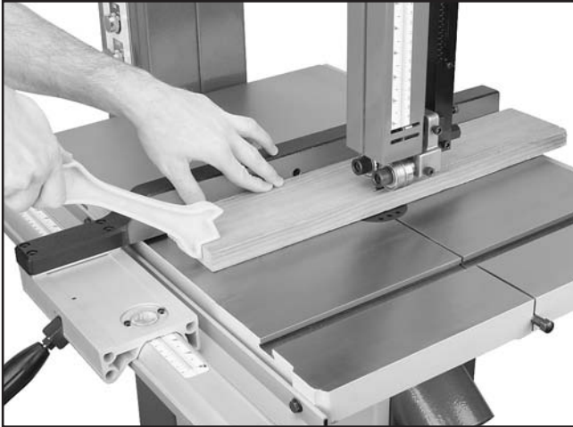
Figure 39. Ripping with a push stick.
