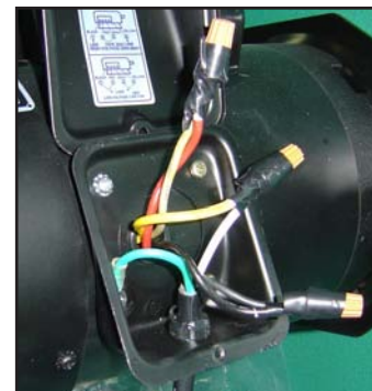
Figure 71. Motor wiring at 220V.
