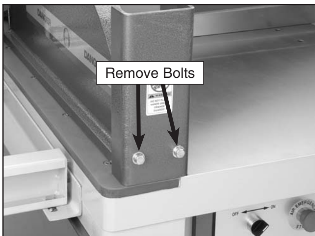
Figure 21. Bolts to be removed for safety guard.
