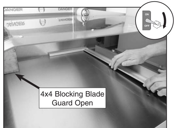
Figure 50. Adjusting fence perpendicular to the blade.
