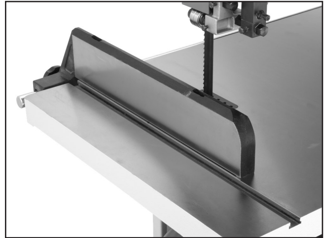
Figure 34. Example of fence square with miter slot.
