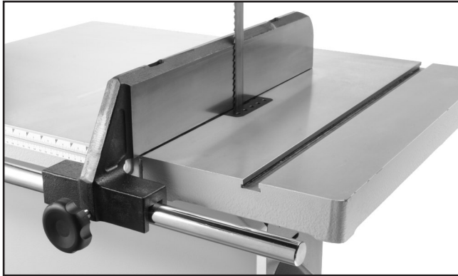
Figure 35. Example of fence flush with blade.
