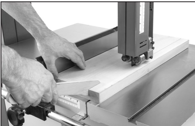
Figure 43. Example of typical ripping operation with a push stick.
