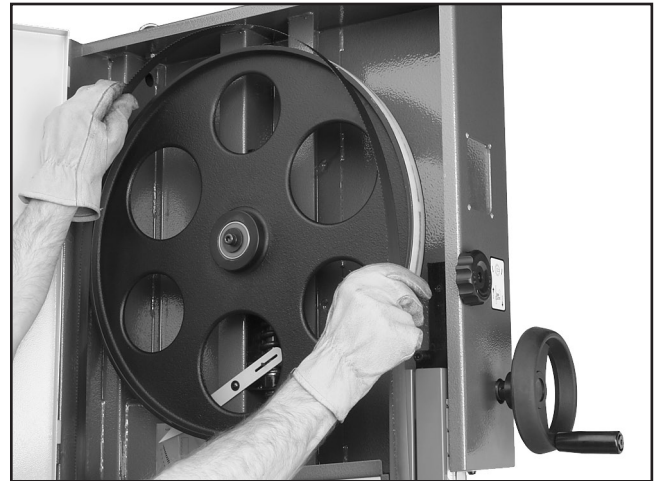
Figure 39. Placing blade on the wheels.
