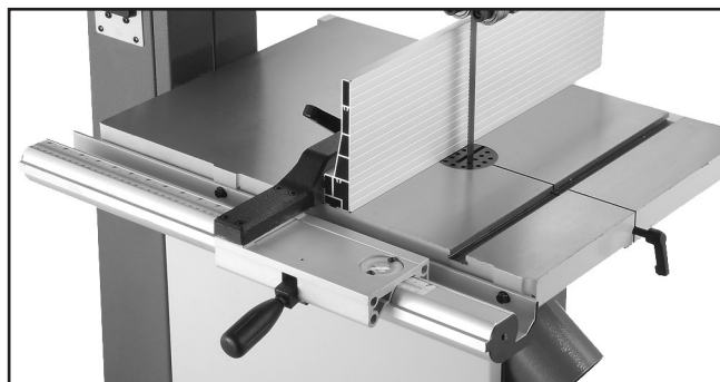
Figure 16. Correctly installed fence.
