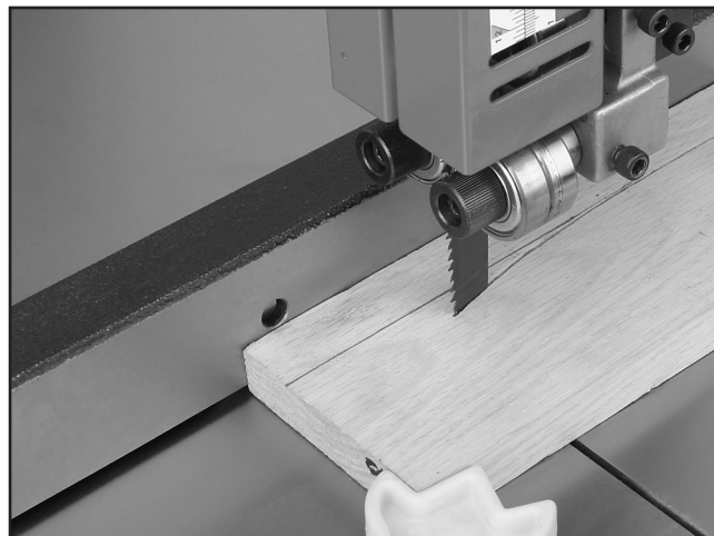
Figure 67. Blade leading away from line of cut.
