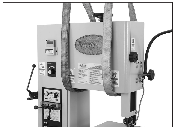
Figure 7. Lifting straps positioned on bandsaw.
