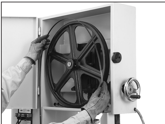
Figure 17. Placing blade on upper wheel.
