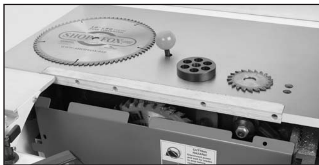
Figure 95. New zero-clearance table insert installed to be cut with a dado blade.
