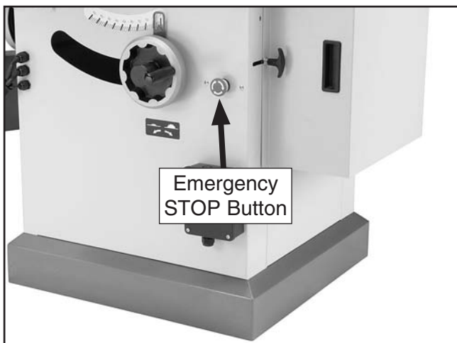
Figure 34. Emergency STOP button.
