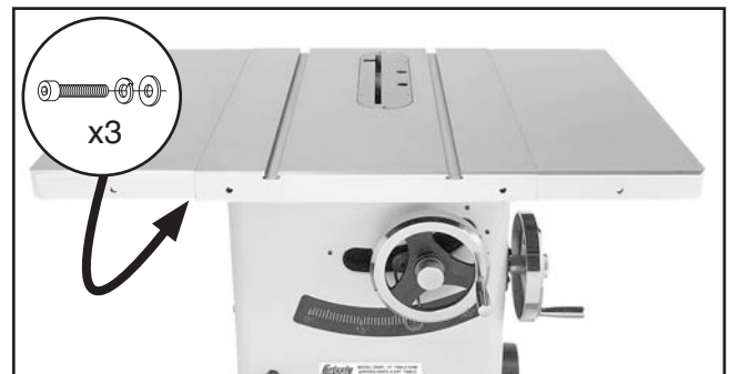
Figure 15. Extension wings installed.
