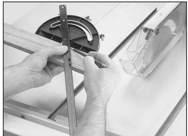
Figure 48. Example of marking miter line.
