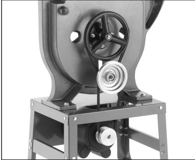
Figure 17. V-belts mounted on pulleys.
