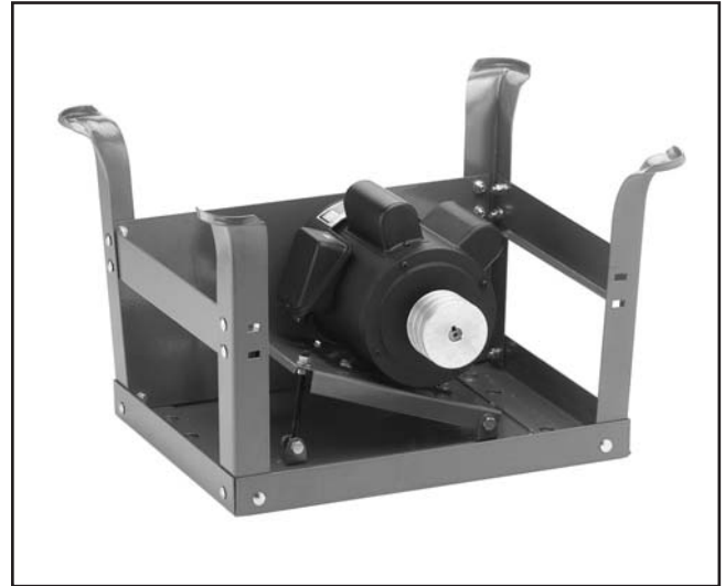
Figure 7. Legs, braces, and one stand side attached to stand
