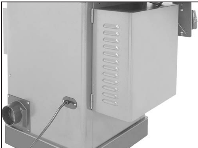
Figure 19. Motor cover installed.
