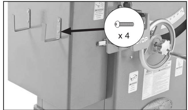
Figure 20. Fence resting brackets installed.
