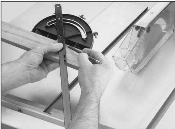
Figure 44. Marking miter line.
