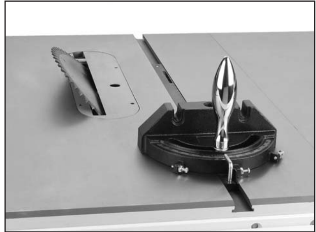
Figure 45. Blade tilted to 45° for bevel cutting on a typical table saw.
