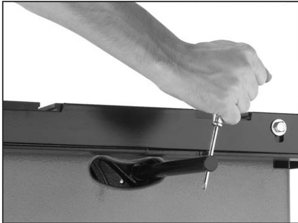
Figure 26. Attaching guard support shaft.
