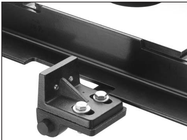
Figure 27. Splitter bracket installed.
