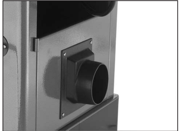
Figure 23. Dust port installed on cabinet.
