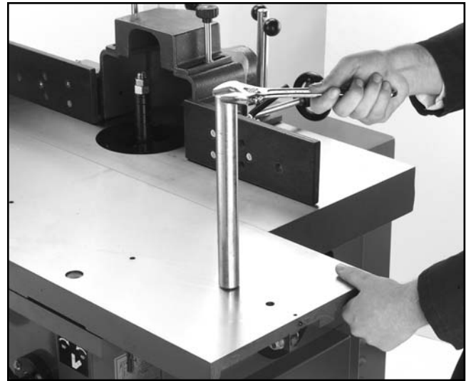
Figure 19. Installing the push shaft.
