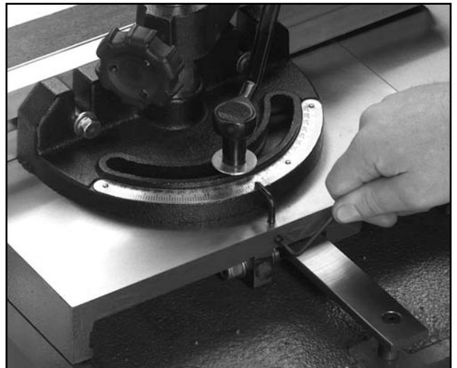
Figure 29. Setting the miter gauge pointer.
