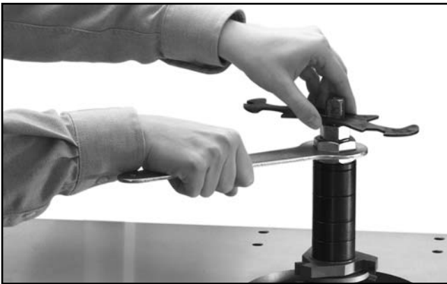
Figure 31. Tightening spindle nuts.
