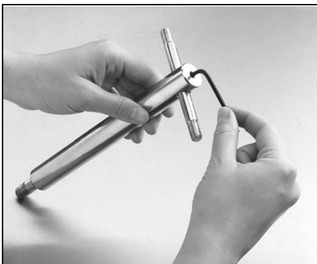
Figure 9. Tightening setscrew with hex key.
