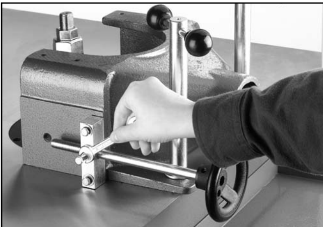
Figure 13. Tightening bolt into shaft groove.
