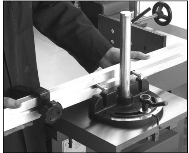
Figure 23. Installing the miter fence.
