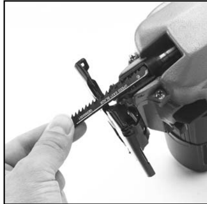
Fig 4. Inserting blade into plunger.
