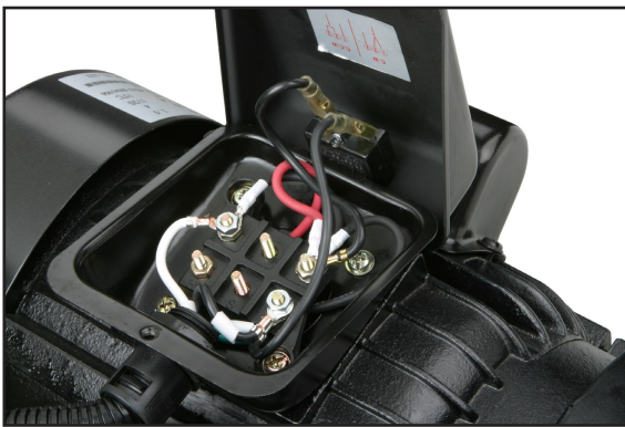
Figure 48. Junction box (M1).
