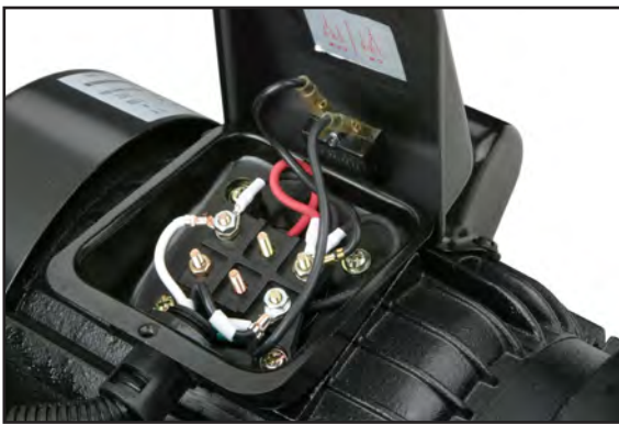
Figure 48. Junction box (M1).
