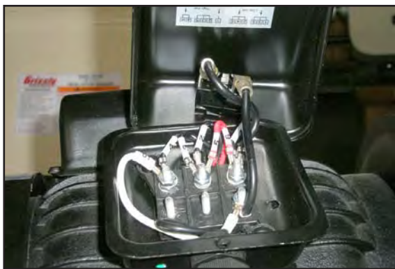
Figure 48. Junction box (M1).
