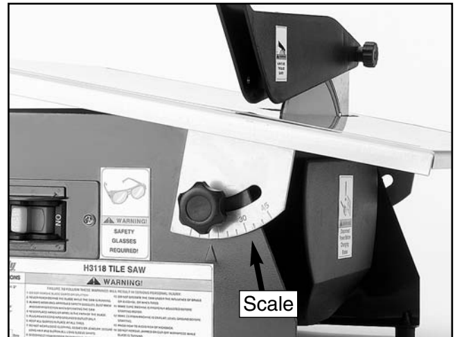
Figure 9. Tilting the table for bevel cutting.
