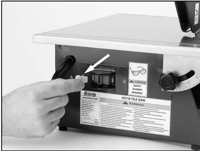
Figure 5. Removable safety key for the power switch.
