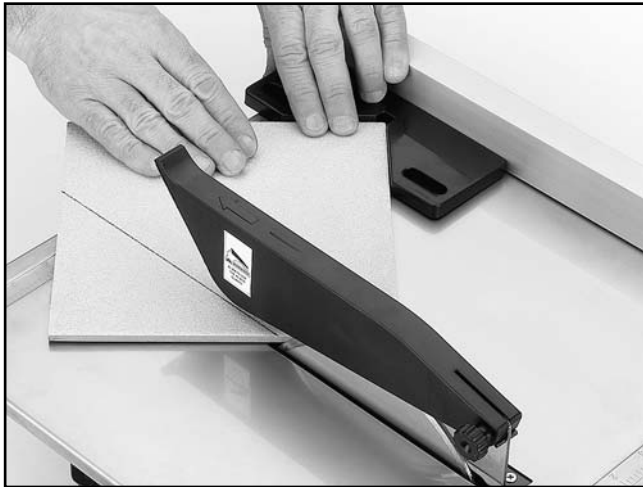
Figure 8. Diagonal cutting with the miter gauge.
