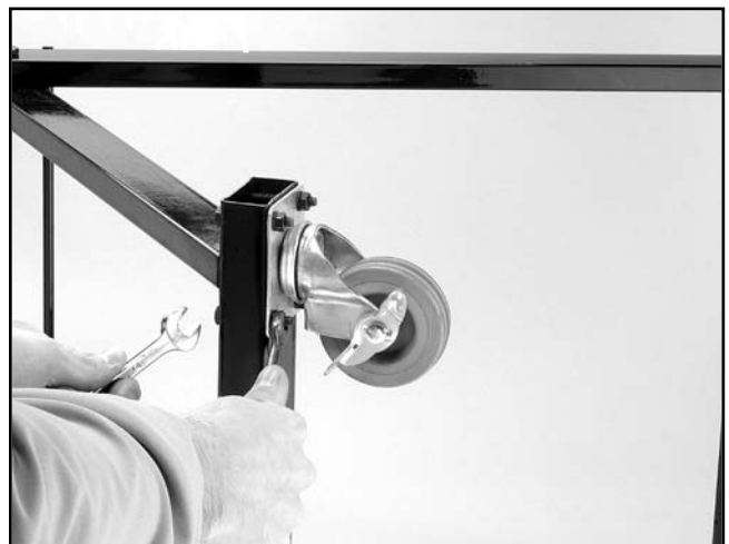
Figure 5. Attaching the casters.
