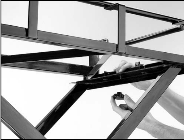
Figure 6. Mounting the saw frame to the stand.
