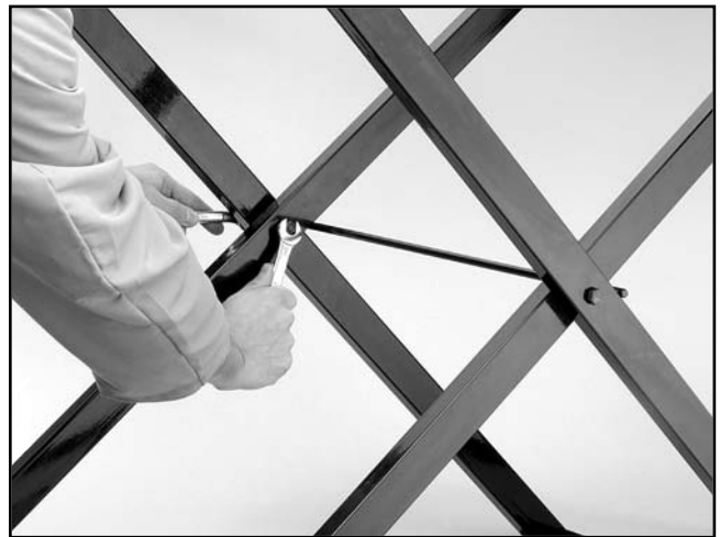
Figure 4. Assembling the stand brackets.
