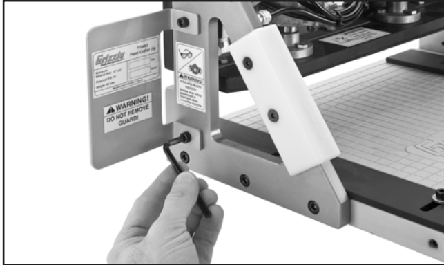
Figure 4. Attaching guard to jig.
