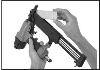
Figure 3. Example of inserting staples into magazine.
