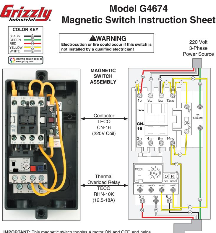
**IMPORTANT:** This magnetic switch toggles a motor ON and OFF, and helps provide thermal overload protection for the motor if operating temperature gradually increases due to heavy work loads. The thermal overload relay inside is not designed to cut power in the event of a sudden motor overload or stall.
