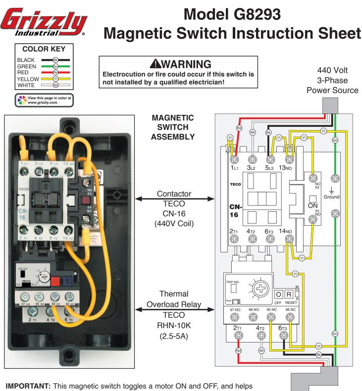
**IMPORTANT:** This magnetic switch toggles a motor ON and OFF, and helps provide thermal overload protection for the motor if operating temperature gradually increases due to heavy work loads. The thermal overload relay inside is not designed to cut power in the event of a sudden motor overload or stall.
