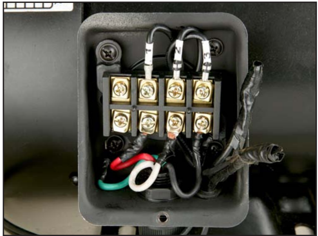
Figure 66. Motor junction box wiring.
