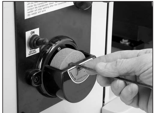
Figure 33. Using the grinder to square up the blade end.
