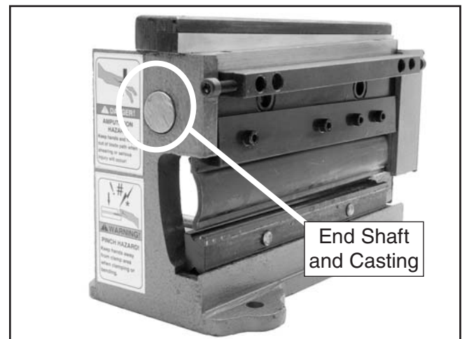
Figure 31. End shaft oil lubrication.
