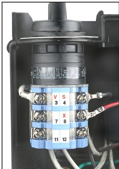
Figure 16. Motor power and direction switch.
