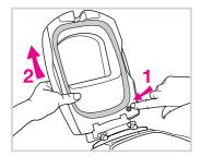
Push on the release button (1) and lift the lid upwards (2).
