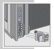
Connect the yellow socket (VIDEO – picture signal) on the television and the corresponding socket on the camcorder (VHS, Video 8) with a cinch cable;
