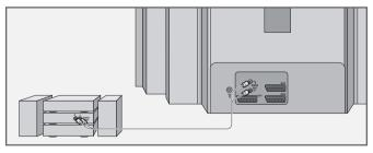
Connect the white and red sockets »L R AUDIO OUT« on the television and the corresponding sockets on the HiFi with a cinch cable.
