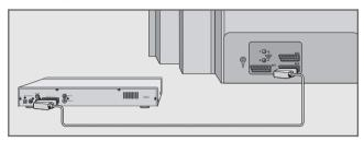
1 Connect the »AV1«, »AV2« or »AV3« television sockets and the corresponding sockets of the video recorder, DVD player or the SET-TOP box with a Euro-AV (Scart) cable.
