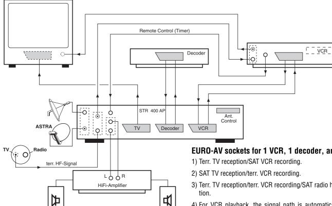
Two aerial systems can be connected to the aerial inputs of the SAT receiver, for example:
