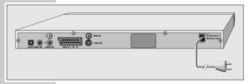
**DIGITAL AUDIO OUT** Audio output socket (optical) for PCM/
