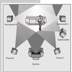
If possible, set up the front loudspeakers in line with the TV set, angled slightly towards the listener. The listener and the speakers should form an equilateral triangle. You thus achieve the best stereo effect.
