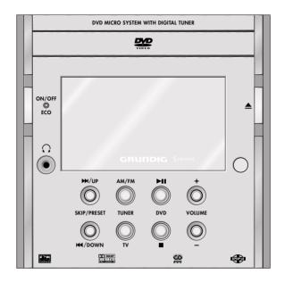
ON/OFF ECO Press briefly: switches the DVD Micro System to standby and back on again with the last source signal selected. Hold down: switches the DVD Micro System from standby to eco mode.
