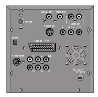
**FM ANT** Connection socket for the FM antenna.
