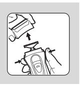
2 Switch on the appliance (in battery mode) and run lukewarm water over the blade units and the detached blade head.
