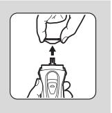
3 Carefully brush hair clippings out of the blades, the inside of the blade head and the housing. Clean the trimmer in the off position.
