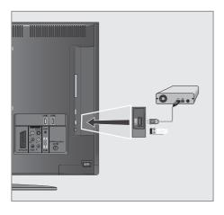
Connect the »USB« socket of the television and the corresponding socket of the data medium (external hard disk) using a USB cable:
