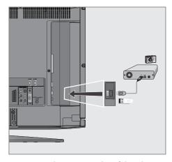
1 Connect the »USB« socket of the television and the corresponding socket on the data device (external hard drive, digital camera, card reader or MP3 player) using a USB cable;
