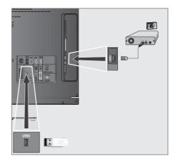
Connect the »USB2 (HDD)« socket of the television and the corresponding socket on the data device (external hard drive, digital camera, card reader or MP3 player) using a USB cable;
