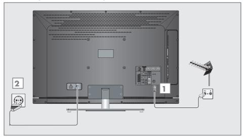
la To receive terrestrial digital broadcasters (DVB-T) connect the cable for the rooftop or indoor antenna (passive or active indoor antenna with its own power supply) to the antenna socket »ANT IN« on the television set:
