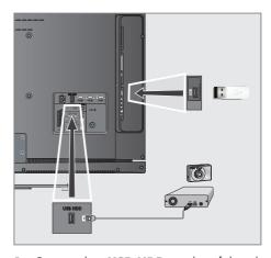
1 Connect the »USB HDD« socket of the television and the corresponding socket on the data device (external hard drive, digital camera, card reader or MP3 player) using a USB cable;
