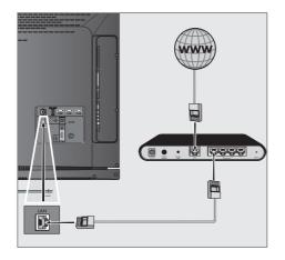
Connect the output of external modem to »LAN« socket with Cat 5 cable.
