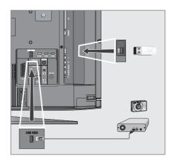
Connect the »USB HDD« socket of the television and the corresponding socket on the data device (external hard drive, digital camera, card reader or MP3 player) using a USB cable;
