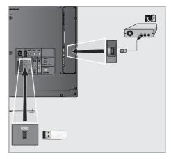
1 Connect the »USB2 (HDD)« socket of the television and the corresponding socket on the data device (external hard drive, digital camera, card reader or MP3 player) using a USB cable;
