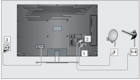
1 To receive digital satellite channels (DVB-S), connect the satellite antenna cable to the antenna socket »SATELLITE« on the television set.
