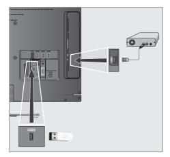
Connect the »USB1« socket of the television and the corresponding socket of the data medium (external hard disk) using a USB cable;
