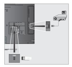
Connect the »USB1« socket of the television and the corresponding socket on the data device (external hard drive, digital camera, card reader or MP3 player) using a USB cable;
