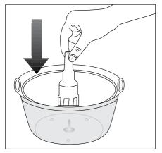
2 Put the shredding attachment ℙ, shredding attachment ⓓ or slicing attachment ◙ on attachment holder ℕ and make sure that it clicks into place.
