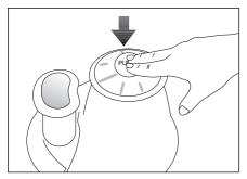
8 Turn the speed control and locking / unlocking button B to the Off position when you want to finish the operation.
