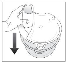
5 Put the base unit A onto the intermediate lid F that is fitted onto the glass bowl I. Make sure that the indicator of the speed control and locking / unlocking button B is at unlock position 1. Turn the indicator of button B to the locked position 1. Make sure that the locking handles D of the base unit are clipped properly onto the handles of the glass bowl I.
