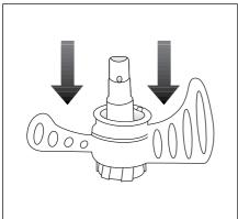
2 Place the accessory support K with the whisk M onto the fixed shaft J in the glass bowl 1.
