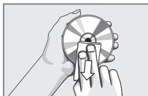
If the device is unable to scan CDs perfectly, use a standard, commercially available cleaning CD to clean the laser optics. Other cleaning methods may damage the laser optics.
