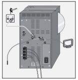
Plug the rooftop antenna cable into the »FM ANTENNA« antenna socket on the hi-fi.
