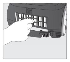
**3** Then remove the sponge filter from the inner area of the air outlet.
