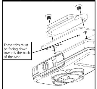
The Universal Locking Plate can be mounted to orient your H2O Audio case in either the up or down orientation, depending on how you would like the case to attach to the mount (as shown).
