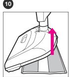
When unit has cooled, remove Ultra-microfiber pad. Store unit upright in a dry area.
