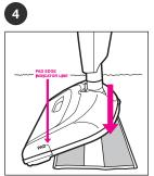
Line up edge of Pad with PAD EDGE INDICATOR LINE. Gently place unit on Ultra-microfiber pad.
