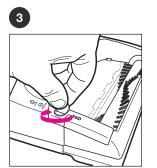
Using a dime, turning clockwise, unlock the brush UNLOCK/LOCK button.
