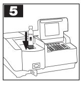
**5**. Zero the instrument using the zero vial (white cap) provided and read the sample.
