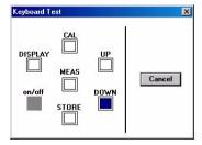
Press any one of the instrument's buttons (**except** the **on/off** button) for a full second or more. The appropriate square on-screen should darken.
