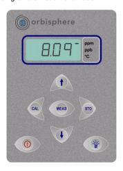
To the LCD's right is a label showing the measurement units configured at the factory for your application.
